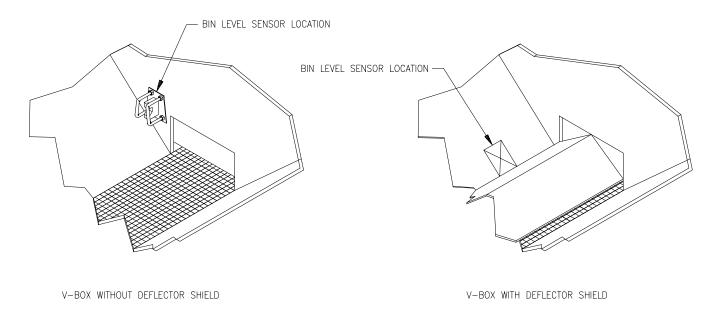
Use the mounting plate as a template to mark the location for the holes. Drill and deburr all holes. Route the sensor cable and secure the mounting plate to the bin wall using U-bolt protectors. Route and connect the sensor cable connector to the flow cable connector. Secure all cables with plastic cable ties.
