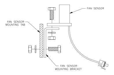
Assemble Fan Sensor to fan sensor bracket with stainless steel bolt, lock washer, and nut. Assemble fan sensor bracket to fan sensor mounting tab on box with stainless steel bolt, lock washer, and nut. (See Figure above).
