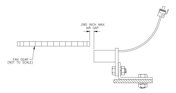
Adjust fan sensor air gap between .040 and .080 inch (.080 inch max.)
